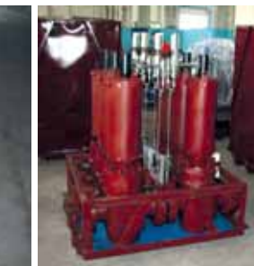
Surface Safety Valve
